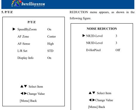
SpeedByZoom: The depth of field scale switch, Optional items: On, Off AF-Zone: Interested in focusing area, Optional
