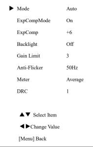
Mode: Exposure mode. Optional items: Auto, Manual, SAE, AAE, Bright ExpCompMode: Exposure compensation mode, Optional items: On, Off (Effective only inAutomode) ExpComp: Exposure compensation value, Optional items:-7 ~ 7(Effective only in ExpCompMode item to on) Gain Limit: Maximum gain limit. Optional Items: 0 ~ 15 (Effective only in Auto, AAE, Bright mode)
