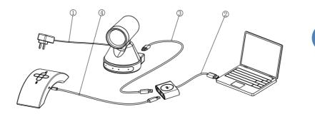
Step1. Please connecting the power adapter to the camera, then Pan-Tilt will self-checking, the lens will lens introspection on the basis of push and pull. When lens and Pan-Tilt self-checking not normal, please confirm whether the power supply to pull plug normal power. If still invalid, please see the specification of the fault phenomenon and processing or phone seeking for technical support.
