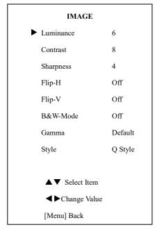
Flip-H: Image flipped horizontally. Optional Items: On, Off. Flip-V: Image Flip Vertical. Optional items: On, Off
